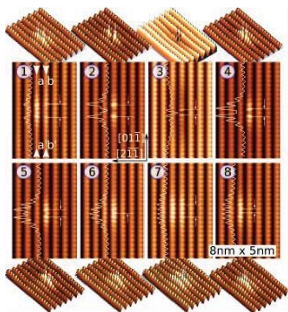
Fig. 1. LDOS( x, y ) maps in vicinity of P atom, located at different positions in subsurface layers of Ge(111)-(2x1) surface. Numbers denote atoms position. Maps are given for zero bias voltage. Profiled along b-b' line are sketched on maps. White lines and arrows are marking the positions of maxima in dimer row, nearest to the impurity atom. Images size is indicated on the figure
